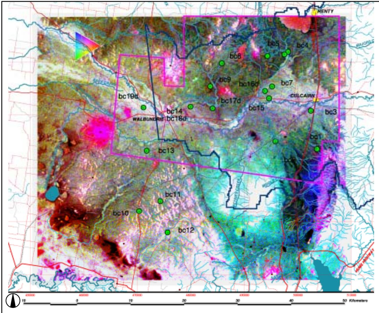
Source: Bureau of Rural Sciences. Horizontal Datum: Geodetic Datum of Australia 1994. Vertical Datum: Australian Height Datum 1971. Green circles—BRS drillholes; magenta line—airborne electro-magnetics boundary; navy blue line—upper Billabong Creek catchment.
