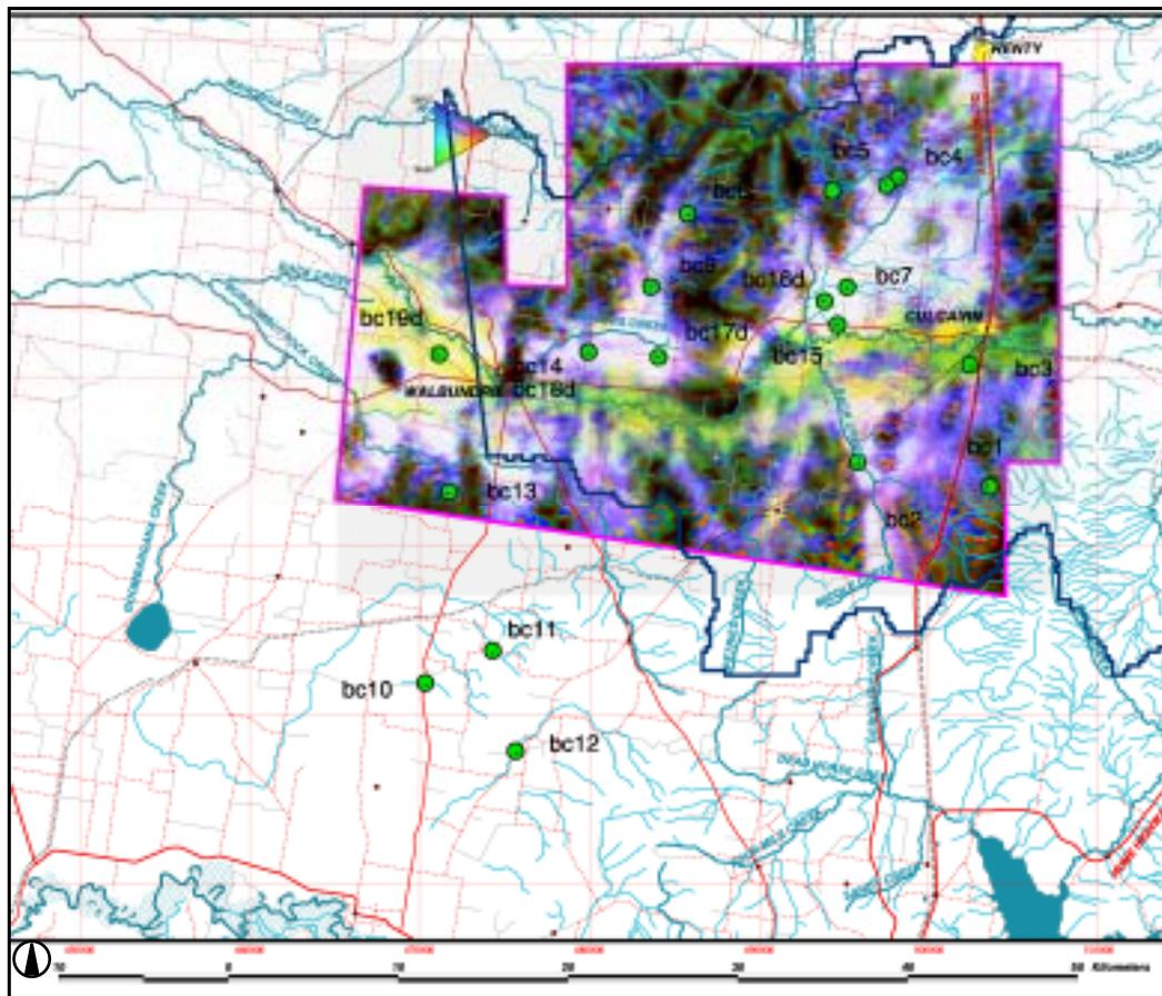
Source: Bureau of Rural Sciences. Horizontal Datum: Geodetic Datum of Australia 1994. Vertical Datum: Australian Height Datum 1971. Green circles—BRS drillholes; magenta line—airborne electro-magnetics boundary; navy blue line—upper Billabong Creek catchment.
