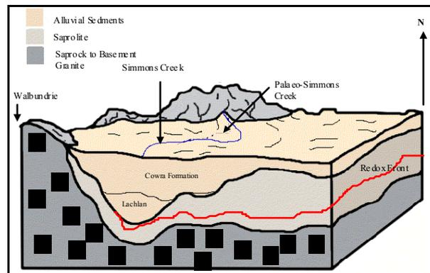
Figure 4. Simmons Creek catchment block model, an example of 3-dimensional hydrogeological modelling.
